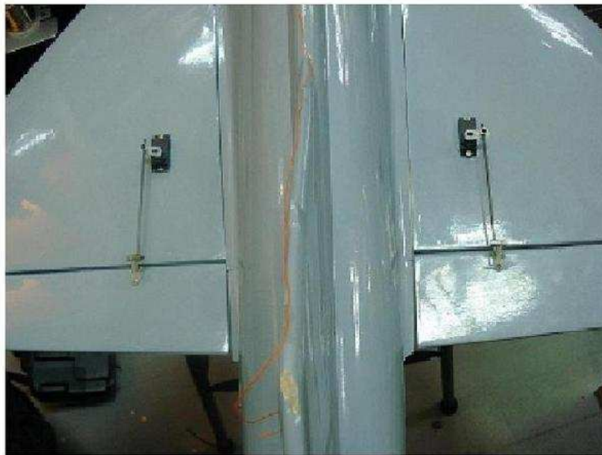
Servos installed to wing with control rods connected.
